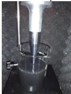
FIGURE 2. Probe sonicator used for preparation of CuO nanofluid
