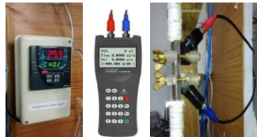
FIGURE 3. Data logger and Ultrasonic flow meter
